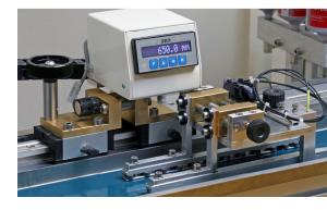
The Metzner ST 25 eccentric drive cutting machine is distinguished by its high cutting capacity and is used for cutting of profiles and tubes in rubber and plastic materials with outstanding precision and repeatability.
